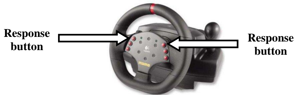
Figure 4.3: Logitech force-feedback steering wheel with associated response buttons (top red buttons on either side of the wheel) [Source: http://support.logitech.com/en_ca/product/momo-racing-force-feedback-wheel ]
