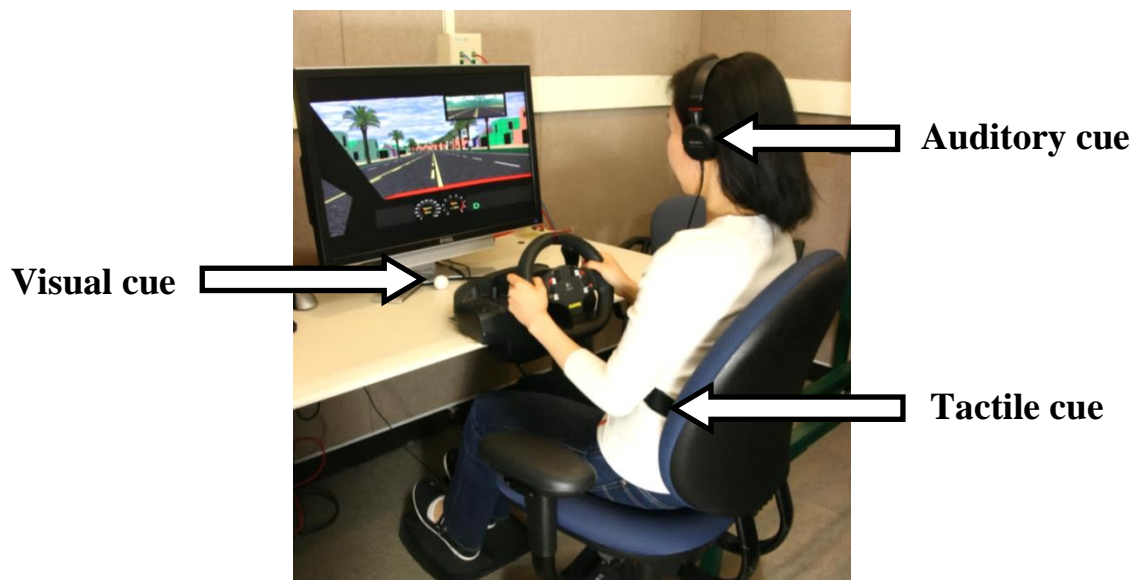
Figure 4.1: Experimental setup (STISIM Drive simulation as background)
