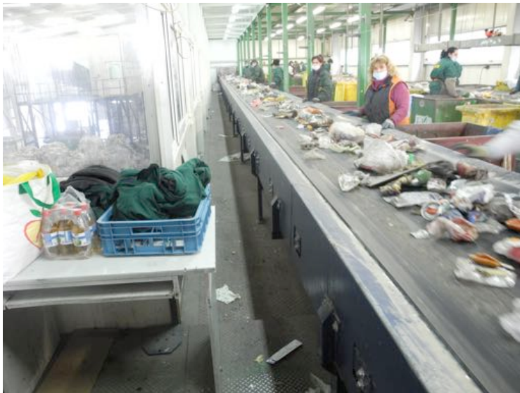
Image 27: Photo of waste conveyor belt: to the left in the glassed-in area is the material for refuse-derived fuel (RDF) and right before that are items that the workers either brought with
