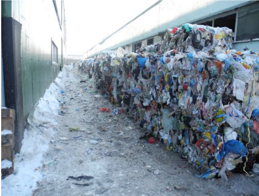
Image 31: Since at the time of research, RDF was only used in one cement plant in Bulgaria, in-process RDF materials were often stored outdoors like this, above. Photo by author.
