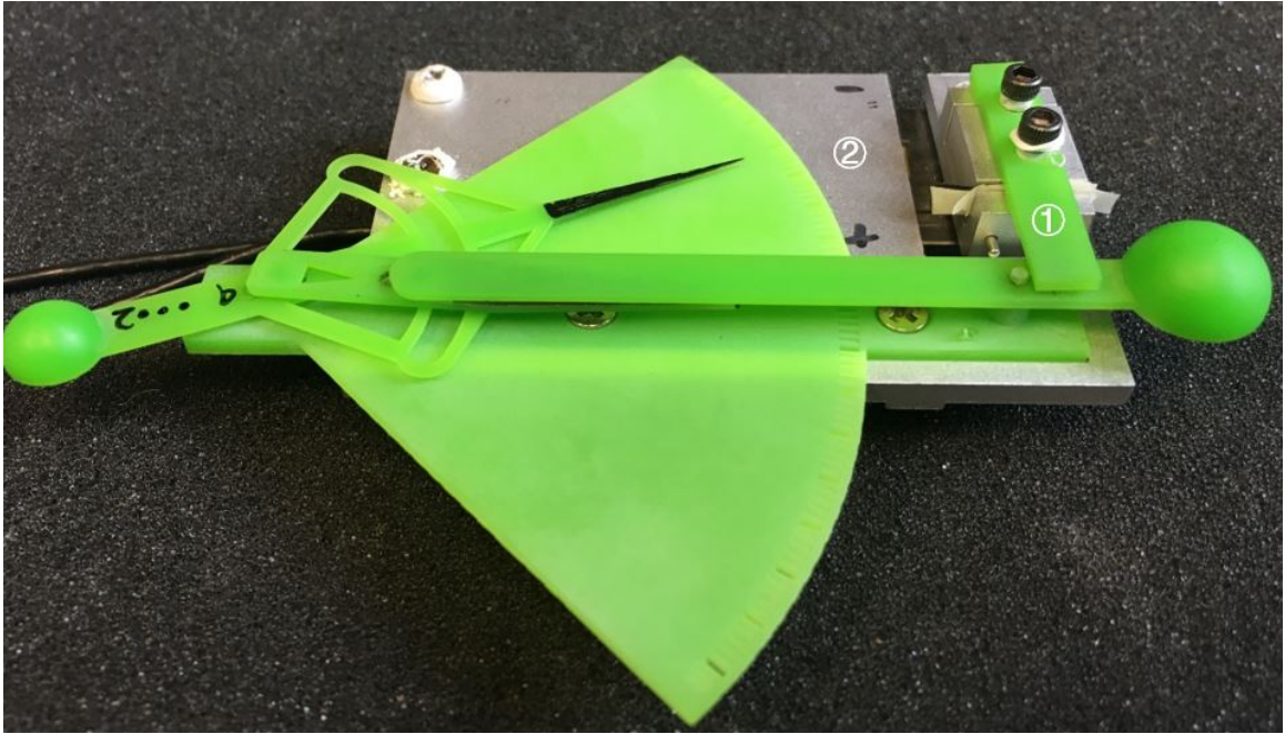
Figure 4.13: SAS with aluminum base on piezo actuator (① Short Sensor Arm ② Aluminum Base)
