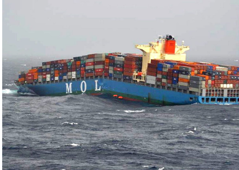
Figure 1.1: MOL Comfort broken in half of the coast of Yemen, June 17, 2013, gCaptain (2014)
