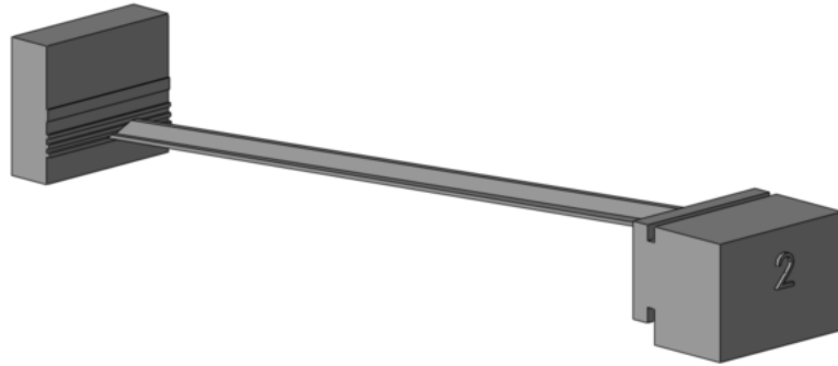
Figure 4.2: PPSS isometric overview. Again with left and right towers with the sensor arm between.
