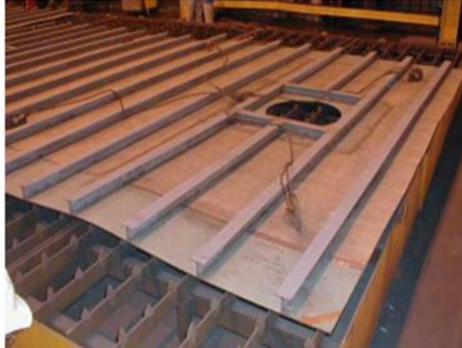
Figure 1.4: welding-induced distortion on a ship panel
