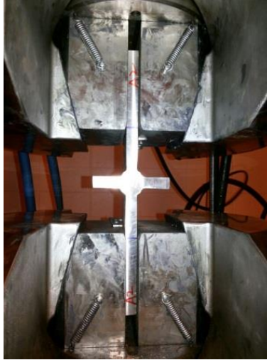
Figure 4.3: A titanium specimen in mounted configuration in hydraulic wedge grips in MTS test machine prior to fatigue testing
