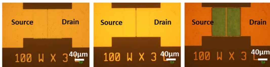
Figure 3-3. Optical micrographs of spin-coated ZTO TFTs of W/L=100\mu\text{m}/3\mu\text{m} with (a) Mo, (b) Au/Ti, (c) ITO source and drain electrodes.
