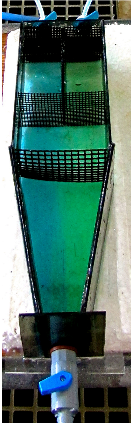
Figure 4.3 Photograph of a dye test highlighting the separation of the two water masses in the two-channel choice flume (left, blue dye; right, green dye)
