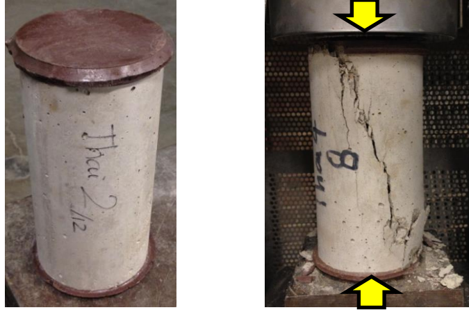
Fig. 3-11: Concrete compressive strength ( f'_c ) measurement (ASTM C39 [118] )
