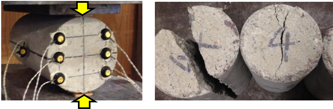
Fig. 3-12: Concrete splitting strength ( f_{ct} ) measurement (ASTM C496 [119] )
