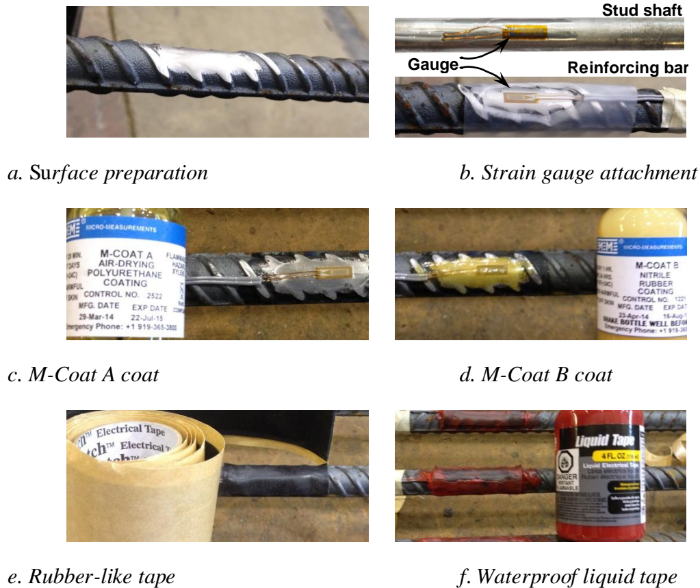
Fig. 3-7: Strain gauge attachment steps
