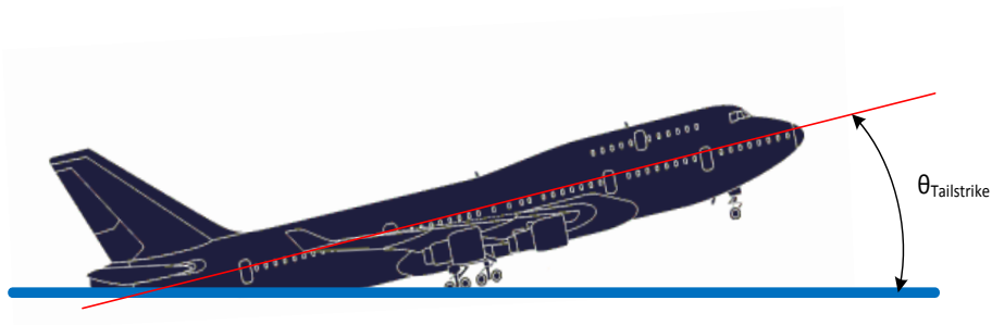
Figure 2.9: Tail strike constraints
