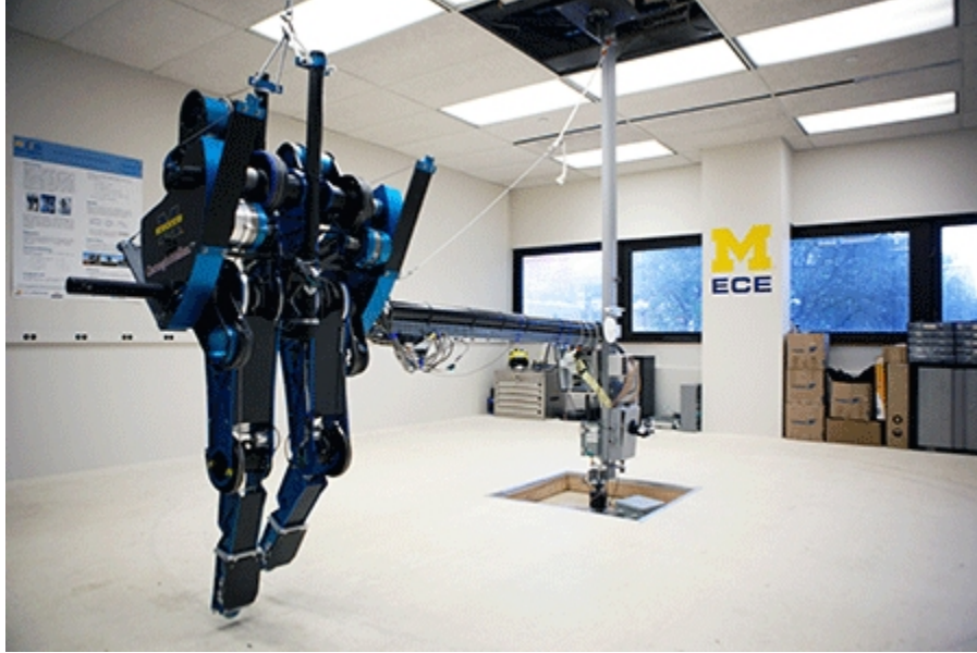
Figure 1.2: The Bipedal Robot MABEL, University of Michigan, 2009. MABEL has reached a pick speed of 3.06 m/s ( Sreenath et al. , 2013).
