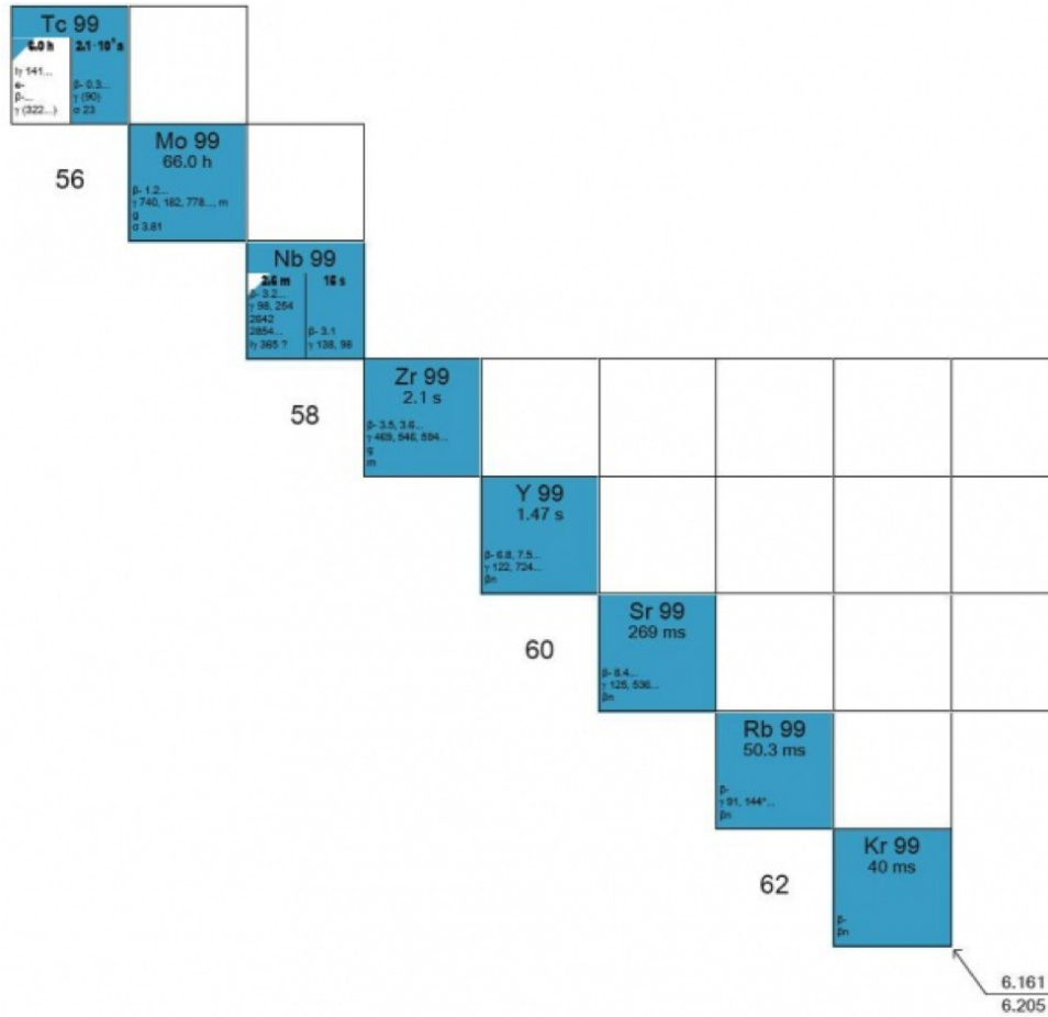
Figure 2.6: Neutron rich isobar chain of atomic weight 99. An example of an isobar chain where beta decay is the primary mode of atomic transition.
