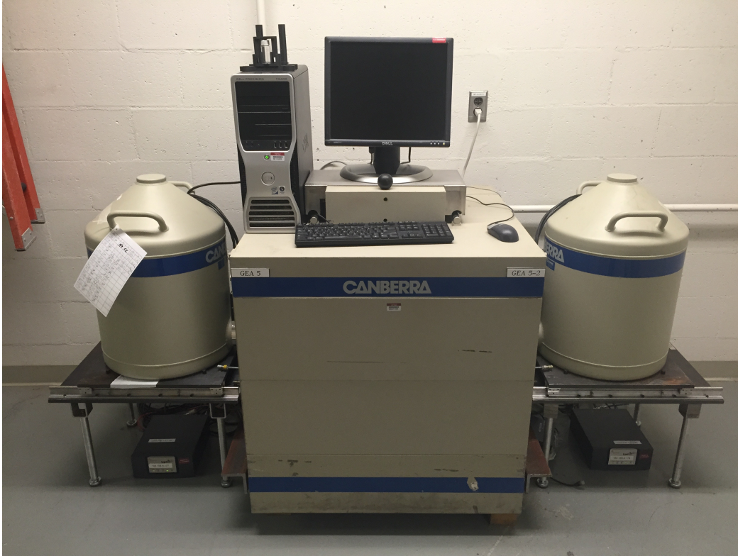
Figure 7.1: HPGe coincidence detector located outside of the LSR of the 318 BLDG.
