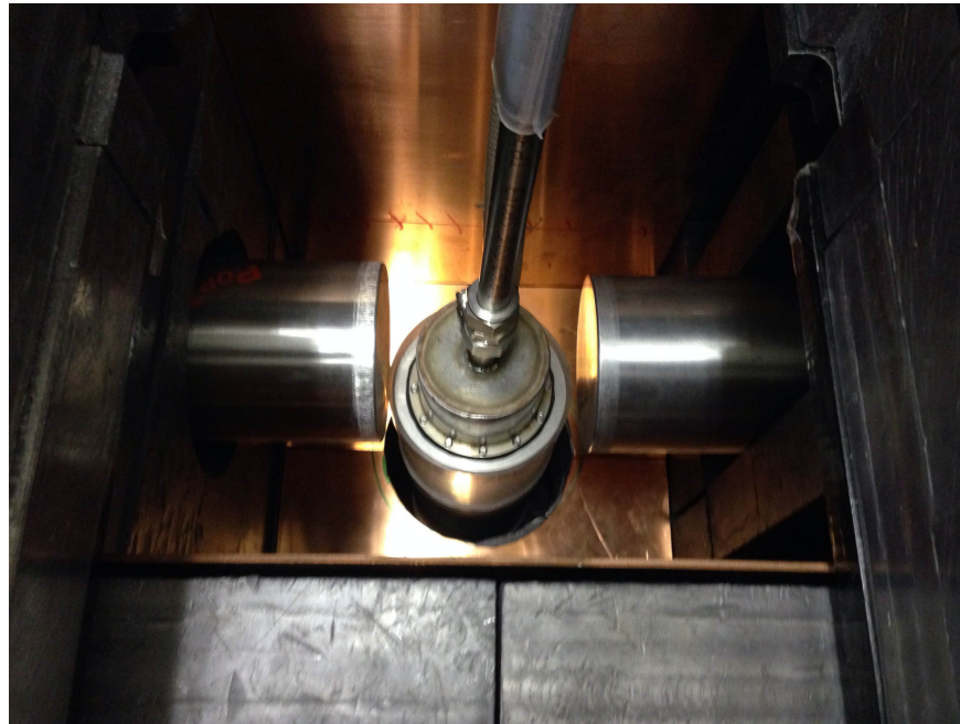
Figure 3.5: HPGe detectors in the lead shield used to acquire data from the experiment. The end station tubing enters through a small hole between the sliding lead doors. Within the lead box are three detectors. Two of the detectors lie roughly along the two cardinal directions and are aptly named east (left in photo) and west. The third detector, named vert, is coupled to the end station using an acrylic spacer. The neutron generator lies several feet north of the detectors behind 2 inches of polyethylene, six feet of concrete, 2 inches of borated polyethylene, 4 inches of lead, and an 1/8" of copper.
