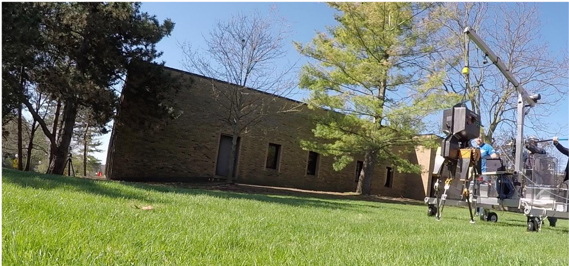
Figure 2.5: MARLO walking on various outdoor terrains. MARLO is able to traverse man-made (top) and natural (bottom) terrain using a single continuously-defined controller based on the mathematical model of the robot. The mobile gantry does not provide any stabilization or support during walking.
