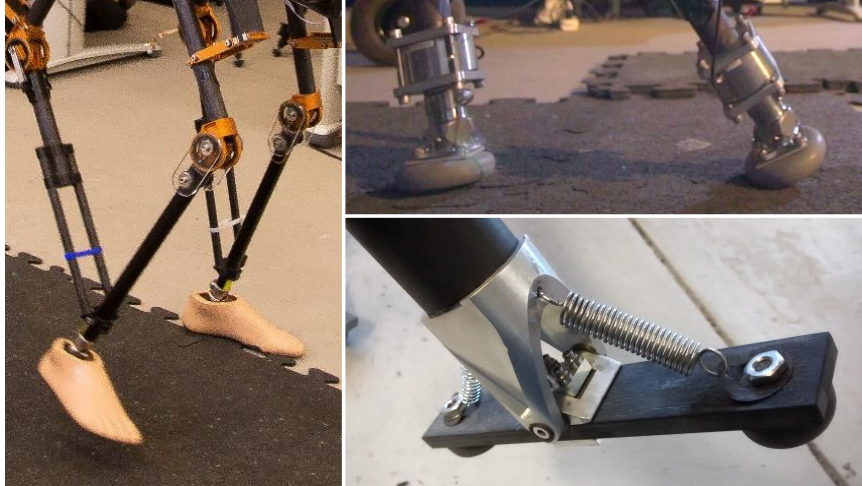
Figure A.11: Foot designs for various levels of yaw restriction. Toroidal feet approximate point feet and provide negligible yaw friction (top right), prosthetic feet add sporadic yaw friction and toe roll (left), and the flexible two-contact-point feet restrict yaw rotation but enable pitch and roll (bottom right).
