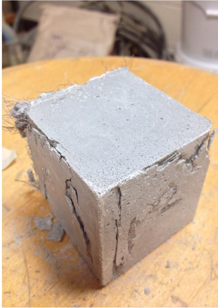
Post Test Compression Specimen
