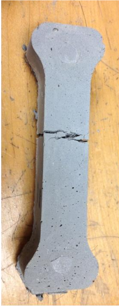
Post Test Tensile Specimen
