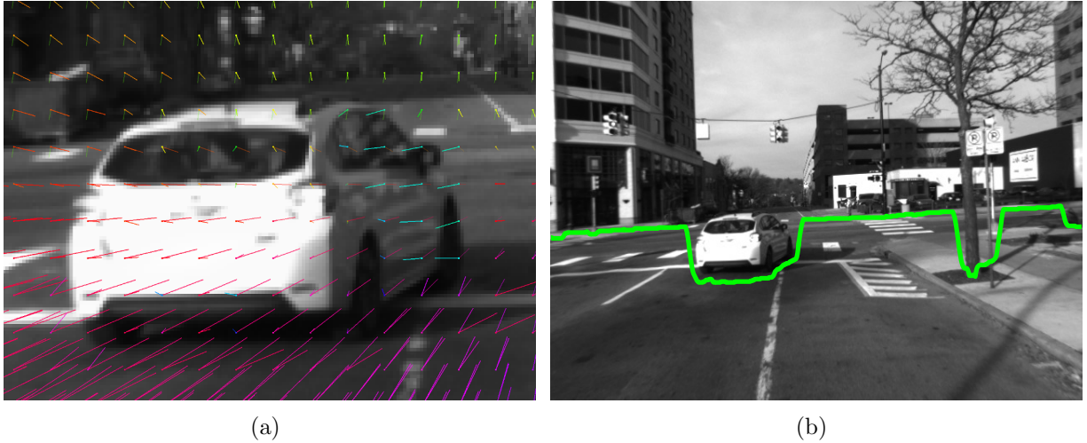
Figure 4.1: In this chapter, we propose to extract optical flow vectors and probabilistically evaluate them against expected flow vectors. We present an MRF framework that fuses various energy potentials, in addition to optical flow likelihood, such that minimizing the energy results in an optimal partition of the image space into ground-map and obstacles, as denoted by the green line through (b).
