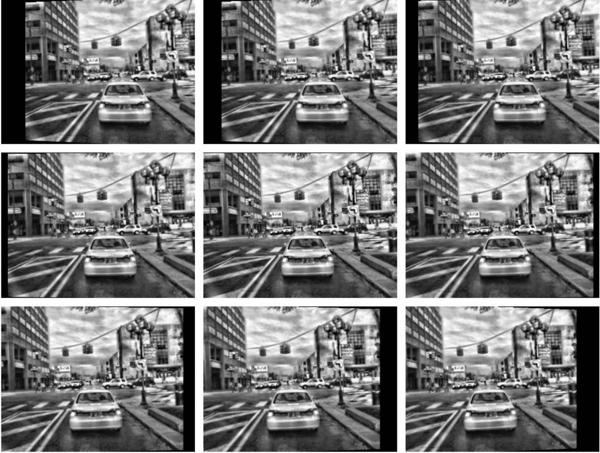
Figure 3.6: Sample warping applied to images to reduce the overall search space for image registration; pictured here are warps of \Delta h = \{-6.0^\circ, -4.5^\circ, -3.0^\circ, -1.5^\circ, 0.0^\circ, 1.5^\circ, 3.0^\circ, 4.5^\circ, 6.0^\circ\} . By rotating each source image in place, we can optimally pull out as much information from a single OpenGL rendered image.
