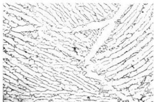
(e) Plate-like acicular \alpha (transformed \beta ); \alpha at prior \beta grain boundaries.
