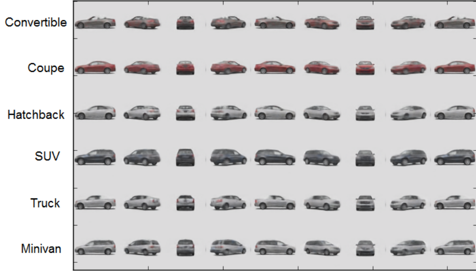
Figure 5.6: Rotations of various body types from the estimated product form design space.
