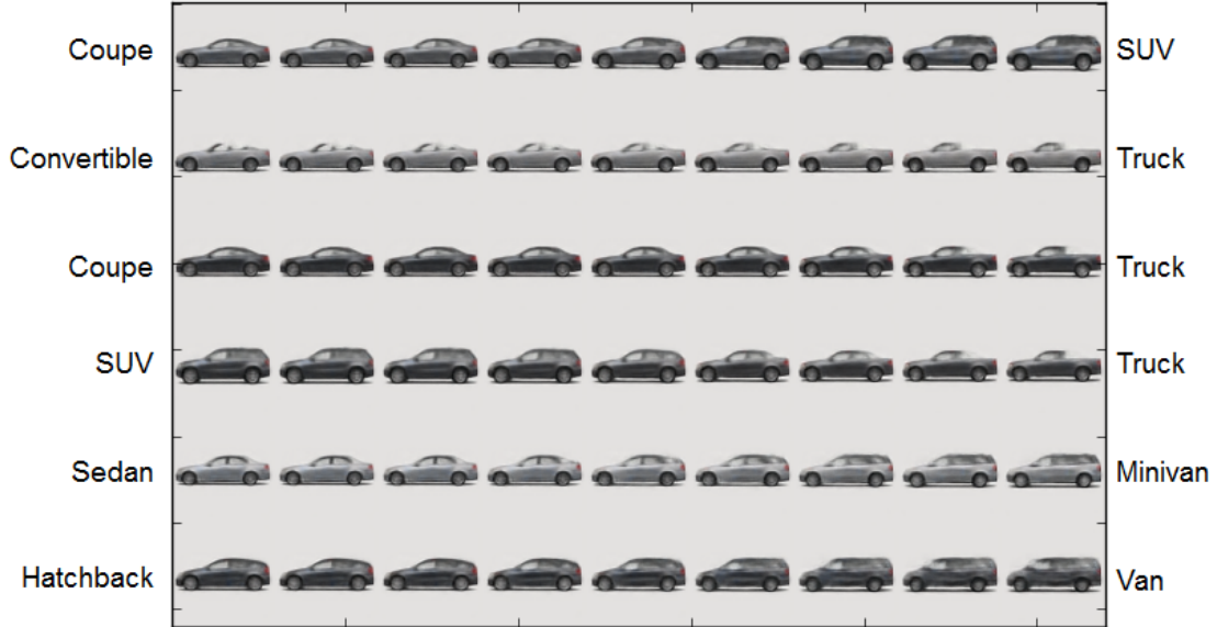
Figure 5.4: Morphing between various body types from the estimated product form design space.
