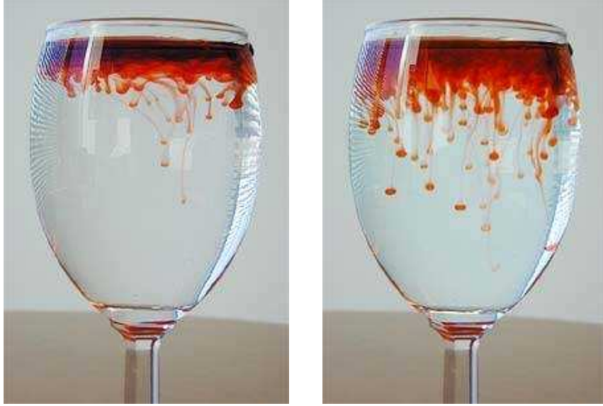
Figure 1.5: Slightly denser dyed water spikes fall in water due to the RT instability. Experimental pictures by James Riordon, AIP.
