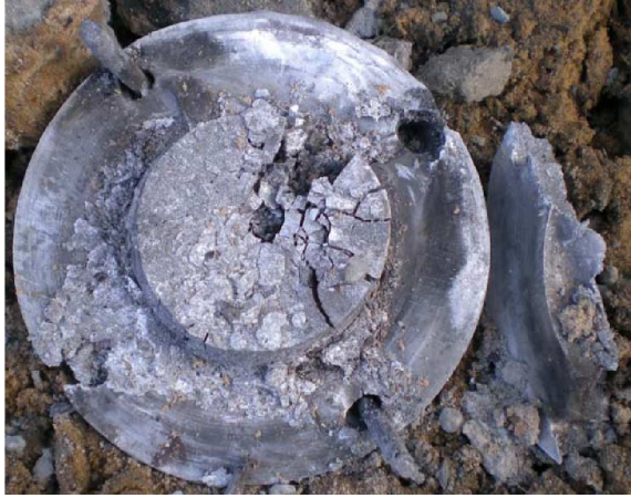
Figure 6.15: Picture of post-shot Be sample loaded with a thin metal impactor.
