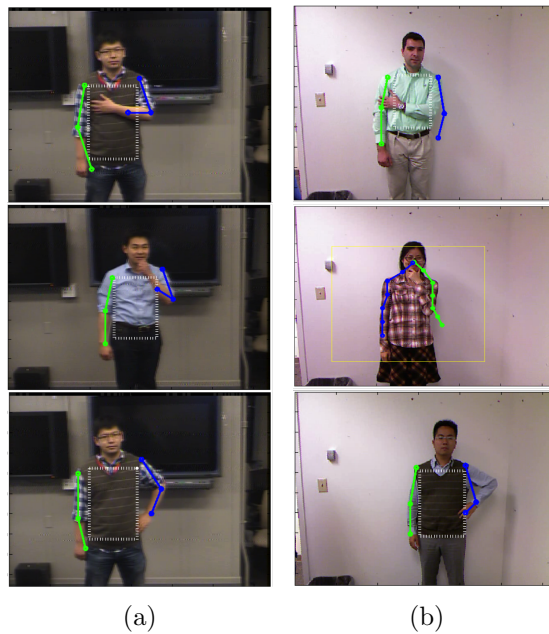
Figure 8.4: Pose estimation comparison between the Smartroom (a) Clean and (b) Noisy datasets for Crossing arms on chest (top), Touching face (center), and Putting arms on hip (bottom) actions. The performance of the MODEC algorithm [199] varies for different clothing and illumination conditions. The Smartroom (Clean) dataset shows more accurate pose estimation than the Smartroom (Noisy) dataset.
