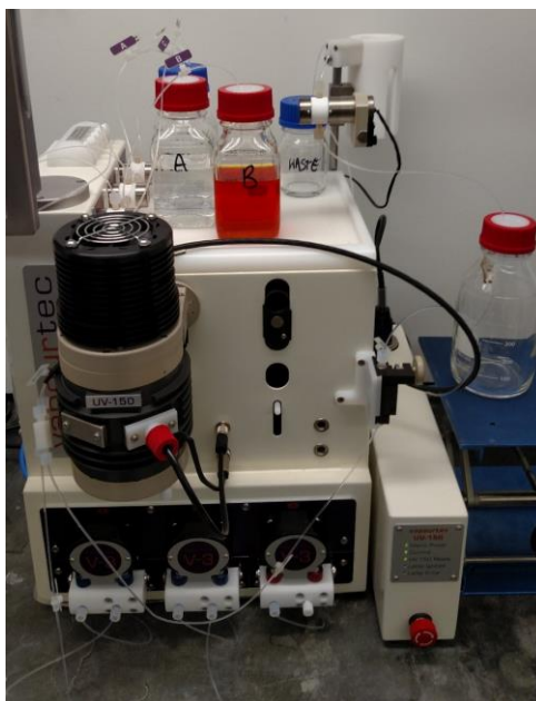
Figure 4.13 Flow apparatus for medium scale trifluoromethylation
