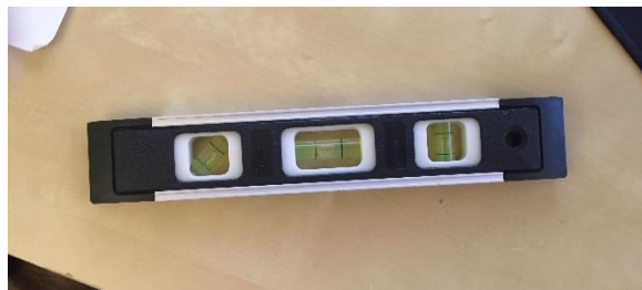
Figure 7.30 The level meter
