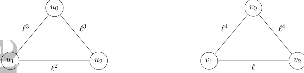
Figure 5: Instance for which the values of near-optimal solutions to k -median, k -tree and k median forest problems are far apart for k = 4 . We have vertex weights q(u_1) = q(u_2) = q(v_1) = q(v_2) = \ell^4 and q(u_0) = q(v_0) = 1 .
