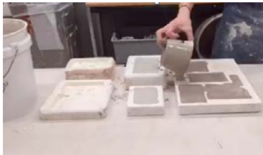
Slip Casting with Plaster molds
