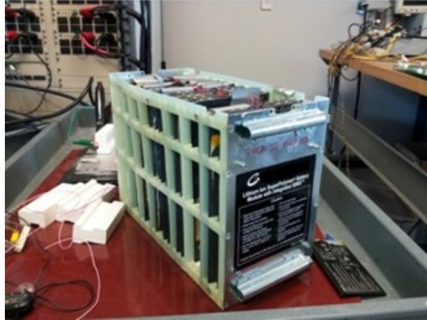
Figure 5.5 Battery pack disassembled from the prototype pickup EV
