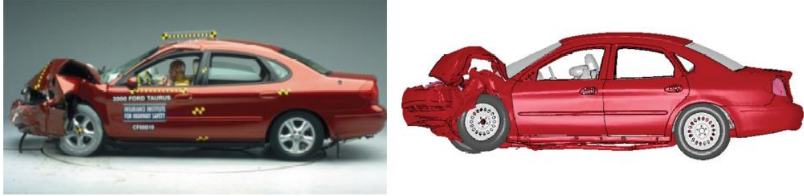
Figure 3.4: Comparison of the full frontal impact between test and model prediction
