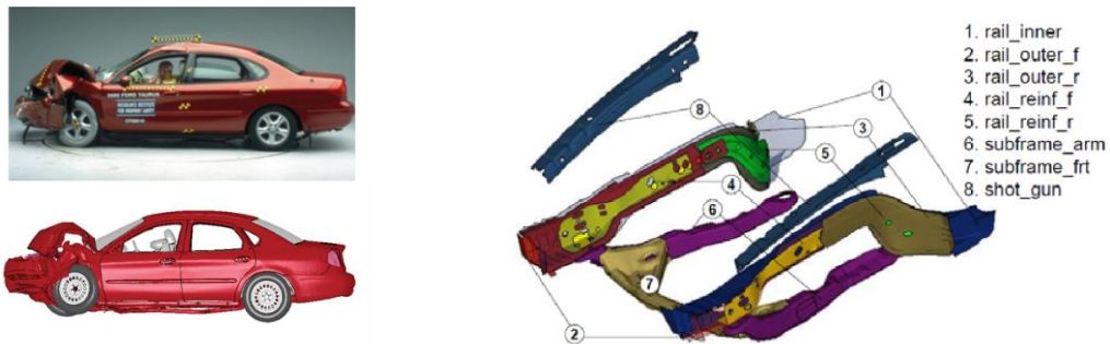
a. Vehicle full frontal impact from test and FEA b. Eight design variables of the main front-end structure
