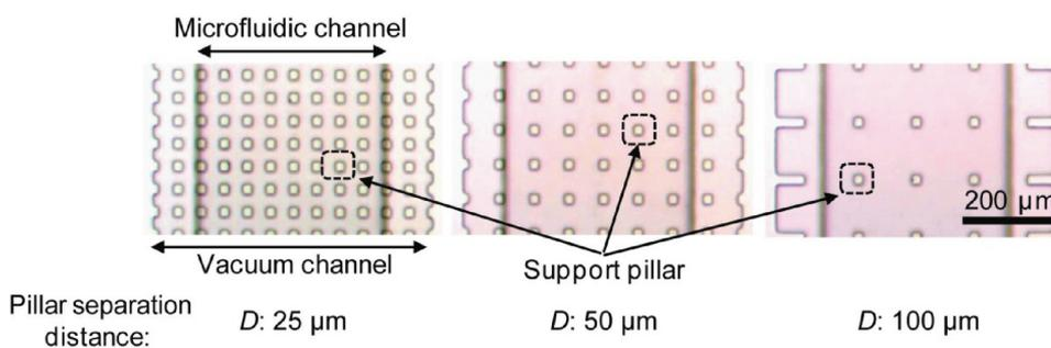
**Figure 2.** Arrays of rectangular support pillars in vacuum channels with the same width  $W$  ( $W = 25 \mu\text{m}$ ) but different separation distances  $D$  ( $D = 25, 50, 100 \mu\text{m}$ ), as indicated.
