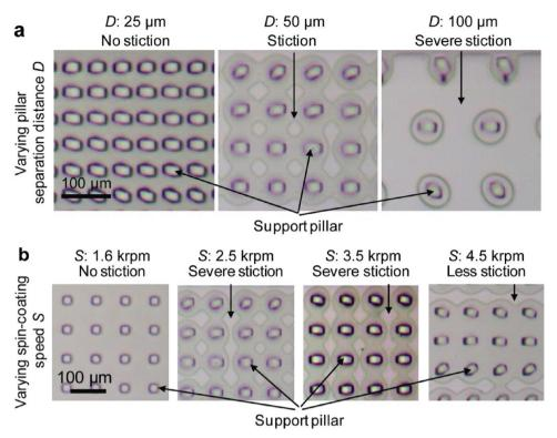
Figure 4. Bright field images illustrating deformation and stiction of thin PDMS membranes to the bottom of vacuum channels when V-PAM was implemented. a) Representative images for support pillar arrays with the same width W but different separation distances D (D = 25, 50, 100  $\mu$ m) as indicated. b) Representative images for thin PDMS membranes generated with different spin-coating speeds S as indicated. D: 50  $\mu$ m. In all cases, P: 12.5 psi, V: 12.5 psi, and W: 25  $\mu$ m.
