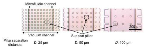
Figure 2. Arrays of rectangular support pillars in vacuum channels with the same width  $W(W=25 \mu m)$  but different separation distances D(D=25, m)50, 100 µm), as indicated.
