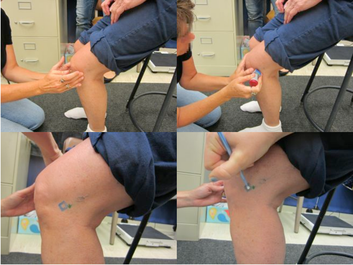
Figure 11. Illustrations of the process of palpating a landmark (upper left), stamping (upper right), marking the corner to digitized (lower left), and marking the contrasting center (lower right).
