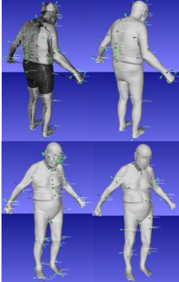
Figure 19. Screenshots from Meshlab showing landmarks extracted from a standing scan in grayscale and surface modes.
