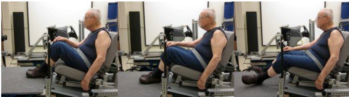
Figure 8. Illustration of the three foot positions used in the passenger mockup: feet back, flat, and on heels.
