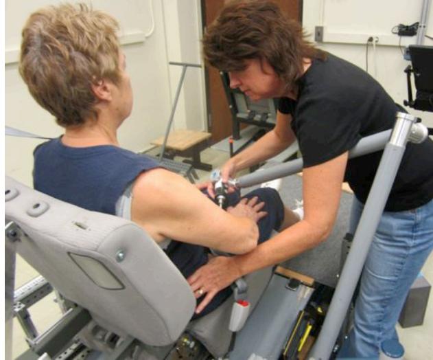
Figure 7. Recording a participant's anterior-superior iliac spine landmark location.
