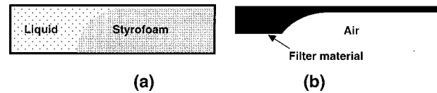
Fig. 3. Schematics of fabricating filters with (a) liquid or (b) solid material.
