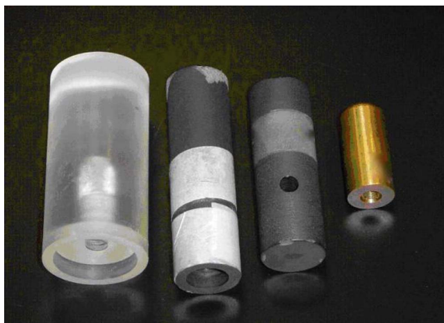
FIG. 9. Recommended miniphantoms for measurement of S_c . The material compositions are, from left to right, Lucite, graphite, and brass. If a high-Z miniphantom is chosen, a correction factor may be required.
