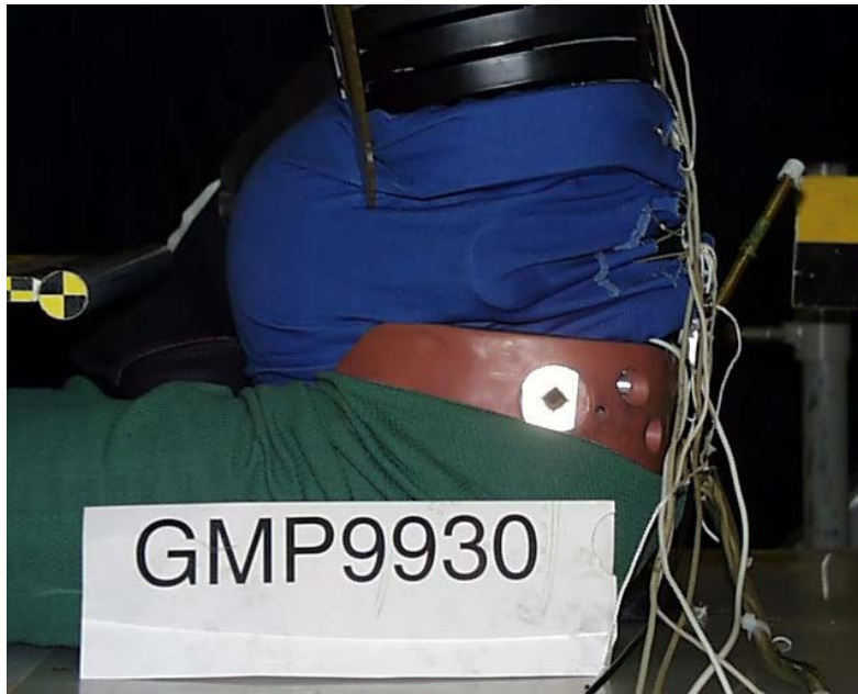
Figure 52. Bladder 6 (40-durometer silicone rubber) with inextensible wrap.
