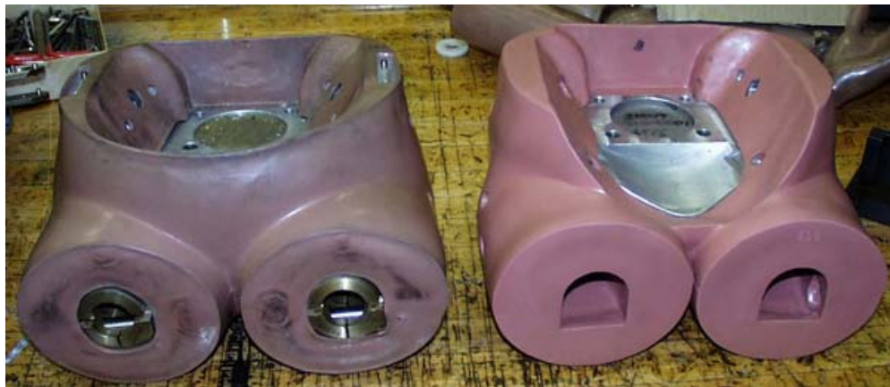
Figure 32. Standard Hybrid III small-female pelvis (left) and first pregnant dummy pelvis (right).
