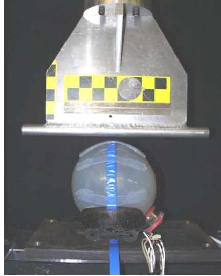
Figure 65. Quasi-static testing of Shape Tape installed in bladder.
