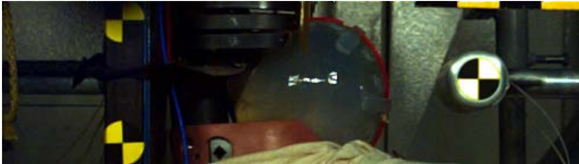
Figure 39. Test setup for surrogate airbag tests showing a side view of the cylindrical impactor (right) and the new pregnant abdomen (center).
