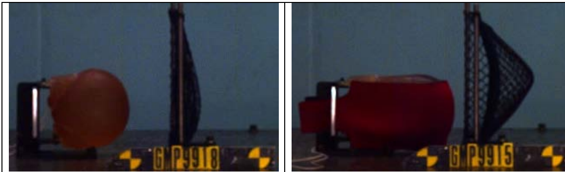
Figure 38. Sled test setup for inertial loading of prototype abdomen showing bladder prior to impact (left) and bladder with jacket material at maximum distention (right).
