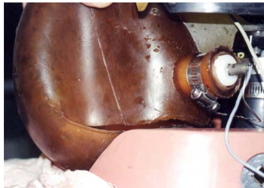
Figure 45. Bladder 2 failure due to shear at lower-mounting cradle during 6-m/s rigid-bar impact.
