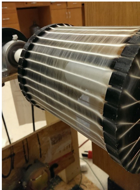
Fig. 1. Photograph of the rotating mandrel set-up for the electrospinning of aligned nanofibers showing the as-spun amorphous fibers aligned across the parallel copper wires on the rotating mandrel.
