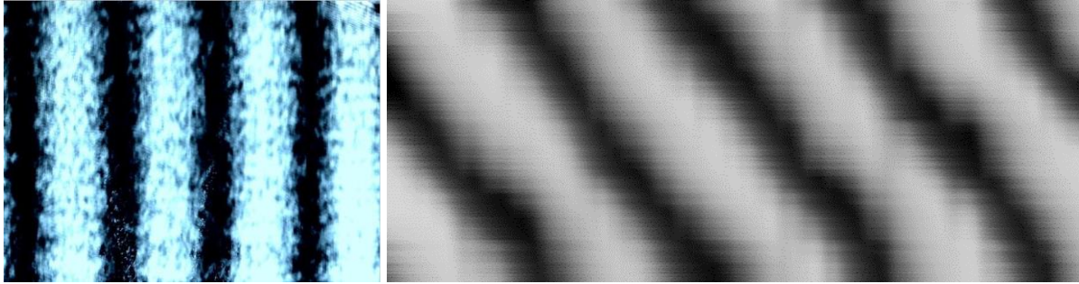
Figure 35. Left: SLM calibration interference fringes, horizontal line along which fringe position was observed. Right: linear response of fringe position to applied voltage. Voltage increasing from minimum to maximum from top of image to bottom.
