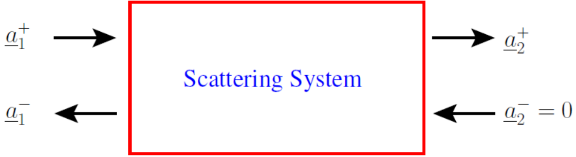
Figure 27. (Jin et al. , 2012) The scattering system used in development of the iterative transmission enhancement algorithm. The scattering sample is assumed to repeat infinitely in the up and down directions. Photons can only enter or leave the system from the right or left. Light incident from the left is set to zero because all incident light is controlled during the experiment. Copyright © 2012 by IEEE.
