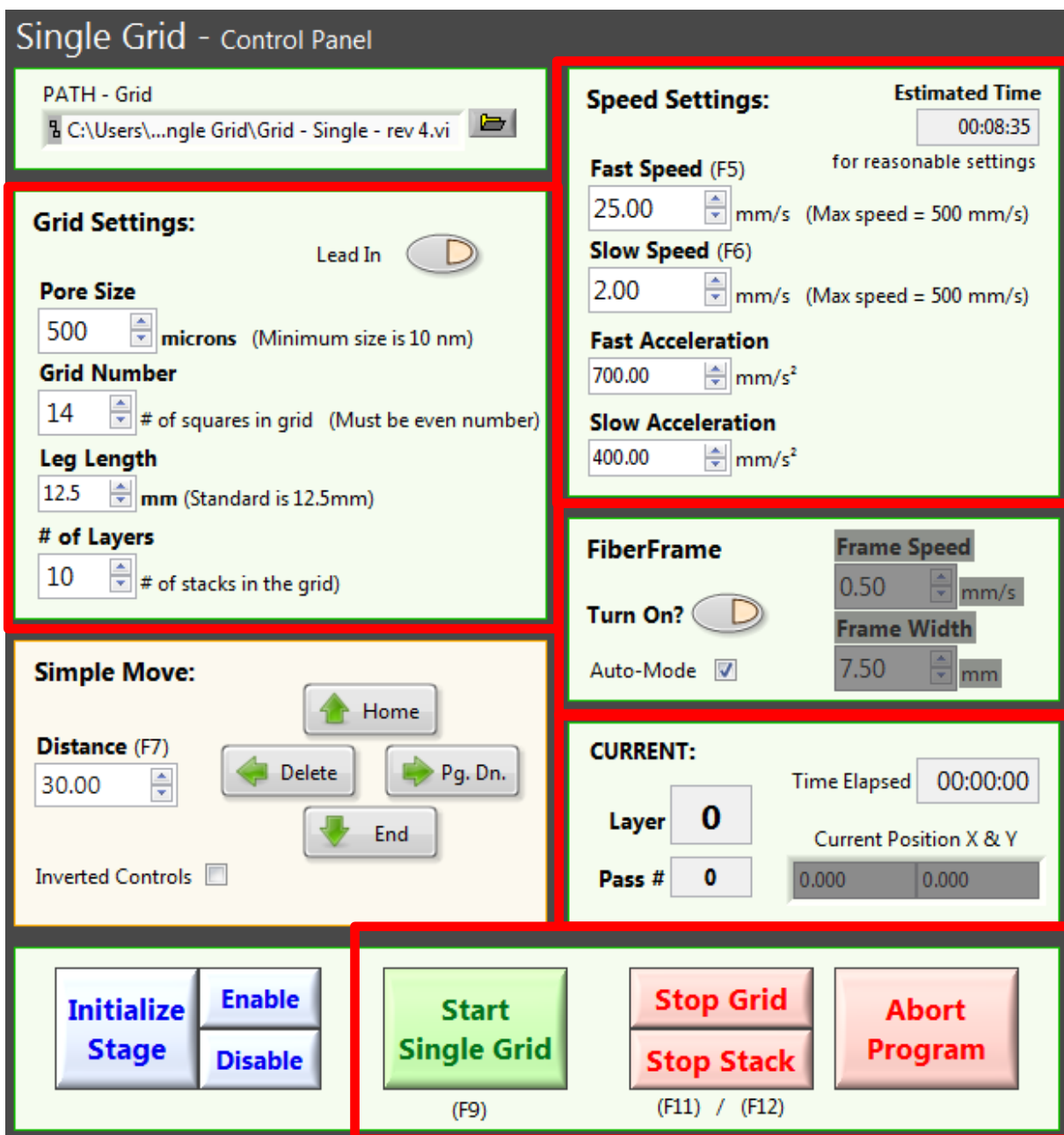
Figure C.1. LabView graphical user interface for scaffold fabrication. The portions of the graphical user interface enclosed in the red rectangles depict the stage controls which are used during scaffold fabrication. In the “Speed Settings” window, the ‘Fast Speed’ and ‘Fast Acceleration’ boxes dictate the speed and acceleration of the stage during the writing of the straight segments of the scaffolds, while ‘Slow Speed’ and ‘Slow Acceleration’ control the speed when changing directions. In the ‘Grid Settings’ window, the pore size, grid number, lead in length, and number of layers of the scaffold are able to be controlled. A coiled fiber fram can be enabled in the ‘FiberFrame’ window. The ‘Current’ window displays the current layer, stack number, and elapsed time of the current scaffold. Scaffold fabrication is started by pressing the ‘Start Single Grid’ button or pressing F9. Stopping the stage movement immediately (Abort Program), at the end of a row (Stop Stack), or at the end of a layer (Stop Grid) are each accomplished at the press of a button or hotkey (F11/F12)
