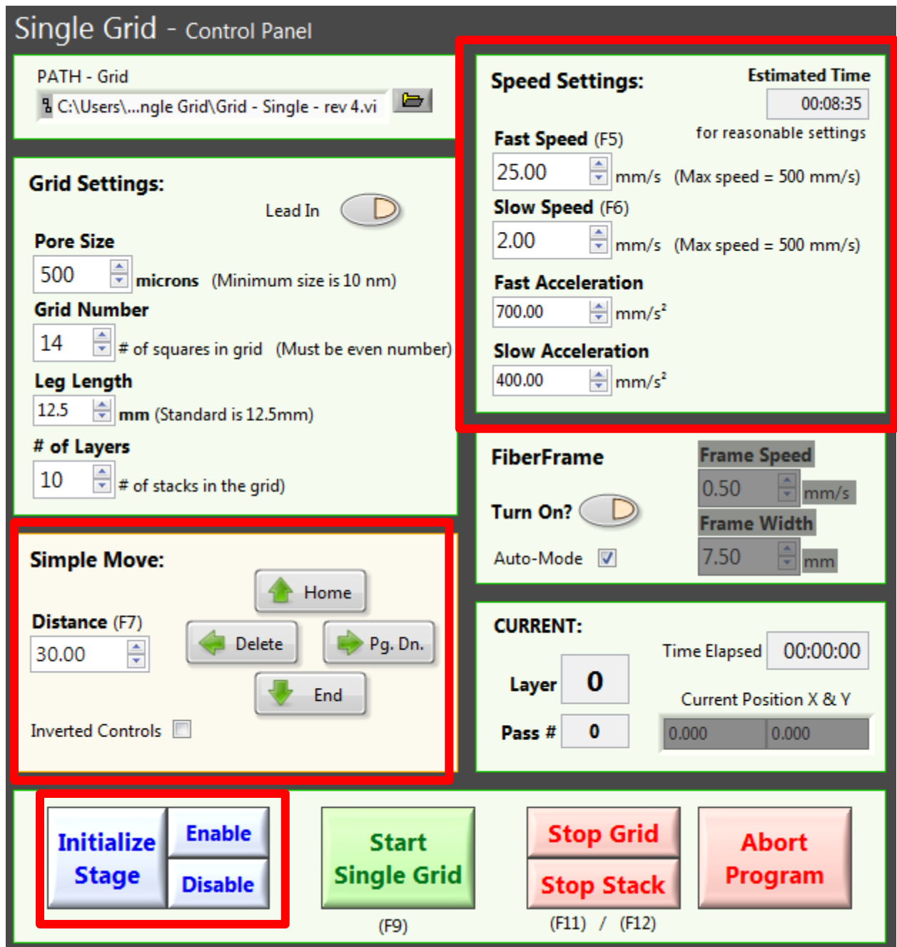
Figure B.2. LabView graphical user interface for stage control prior to scaffold fabrication. The portions of the graphical user interface enclosed in the red rectangles depict the stage controls which are used prior to scaffold fabrication. In the “Speed Settings” window, the ‘Fast Speed’ and ‘Fast Acceleration’ boxes dictate the speed and acceleration of the stage during the manual control mode. The “Simple Move” window has a ‘Distance’ option which allows the user to dictate how far the stage will move for each movement command, with the option of inverting the controls. The up, down, left, and right arrows can be either pressed on the screen via mouse click, or the corresponding keyboard hotkeys can be pressed to move the stage in the desired direction. Initializing the stage is required prior to any controlled movement of the stage, and connection can be disabled or enabled as needed.
