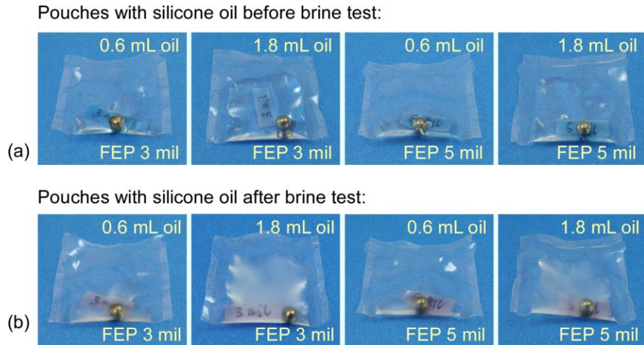
Figure 4.11: Sealed pouches with silicone oil for 3 h boiling brine test: (a) before test; (b) after test. Water vapor permeated into all the pouches, and changed the color of moisture strips into pink.
