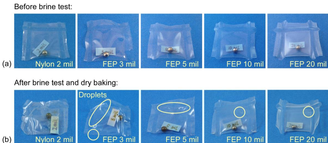
Figure 4.9: Sealed pouches for 3 h boiling brine test followed by dry baking: (a) before test; (b) after test and dry baking. Water vapor permeated into the pouches, and the baking process did not evaporate all the vapor. In the cases of FEP 5 mil, 10 mil, and 20 mil, vapor condensed away from the moisture strip area, and therefore the moisture strip did not change color.
