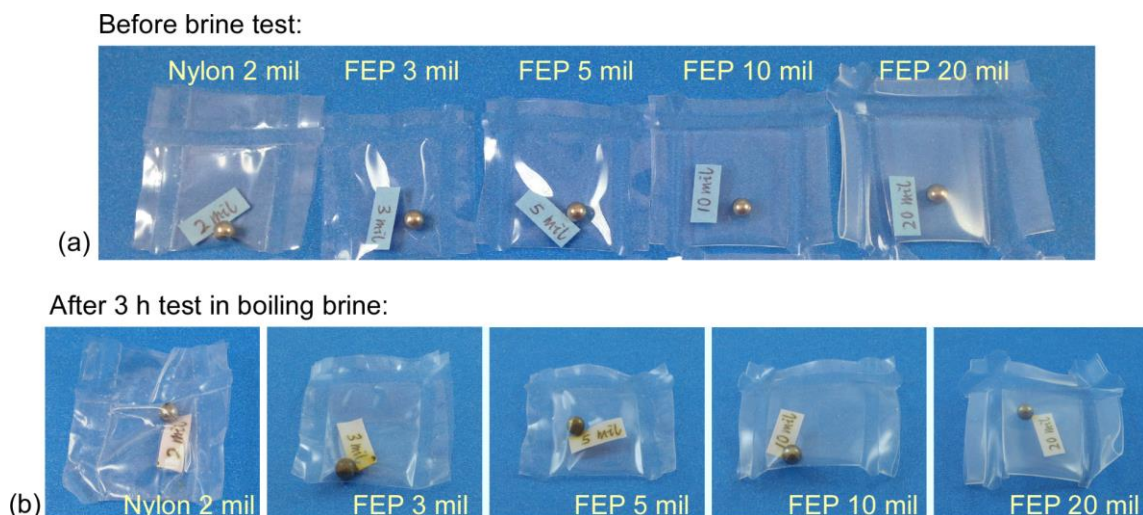
Figure 4.7: Sealed pouches for 3 h brine test at boiling temperature: (a) before test; (b) after test. No degradation in Nylon and FEP after the test. No gross leakage, but water vapor permeated through all films, changing the color of the moisture strips from blue to pink.
