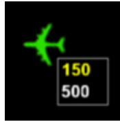
Figure 2.2 - Aircraft icon and data block showing airspeed (150 kts) and altitude (FL (flight level) 500)
