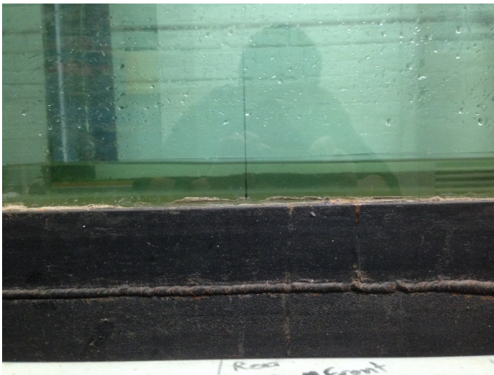
Figure 44: Sample photograph to derive wave profile
