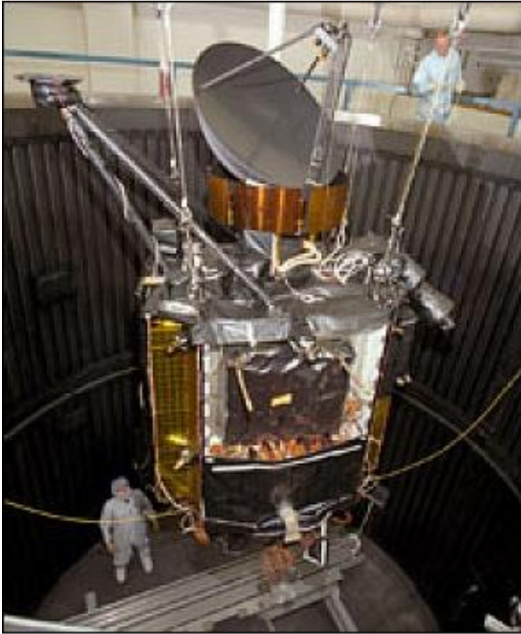
Figure 8: QuickSCAT undergoing tests in a thermal vacuum chamber. Source: https://directory.eoportal.org/web/eoportal/satellite-missions/q/quikscat
