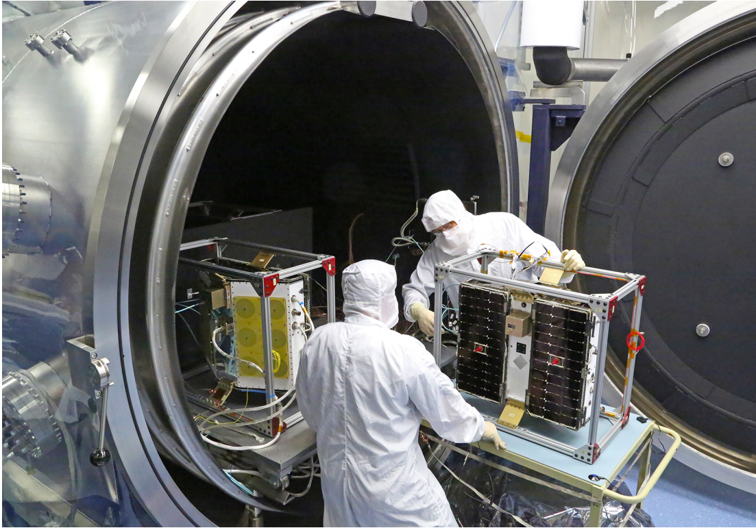
Figure 9 CYGNSS observatories undergoing tests in a thermal vacuum chamber. Source: http://www.nasa.gov/press-release/nasa-invites-media-to-learn-about-new-hurricane-mission
