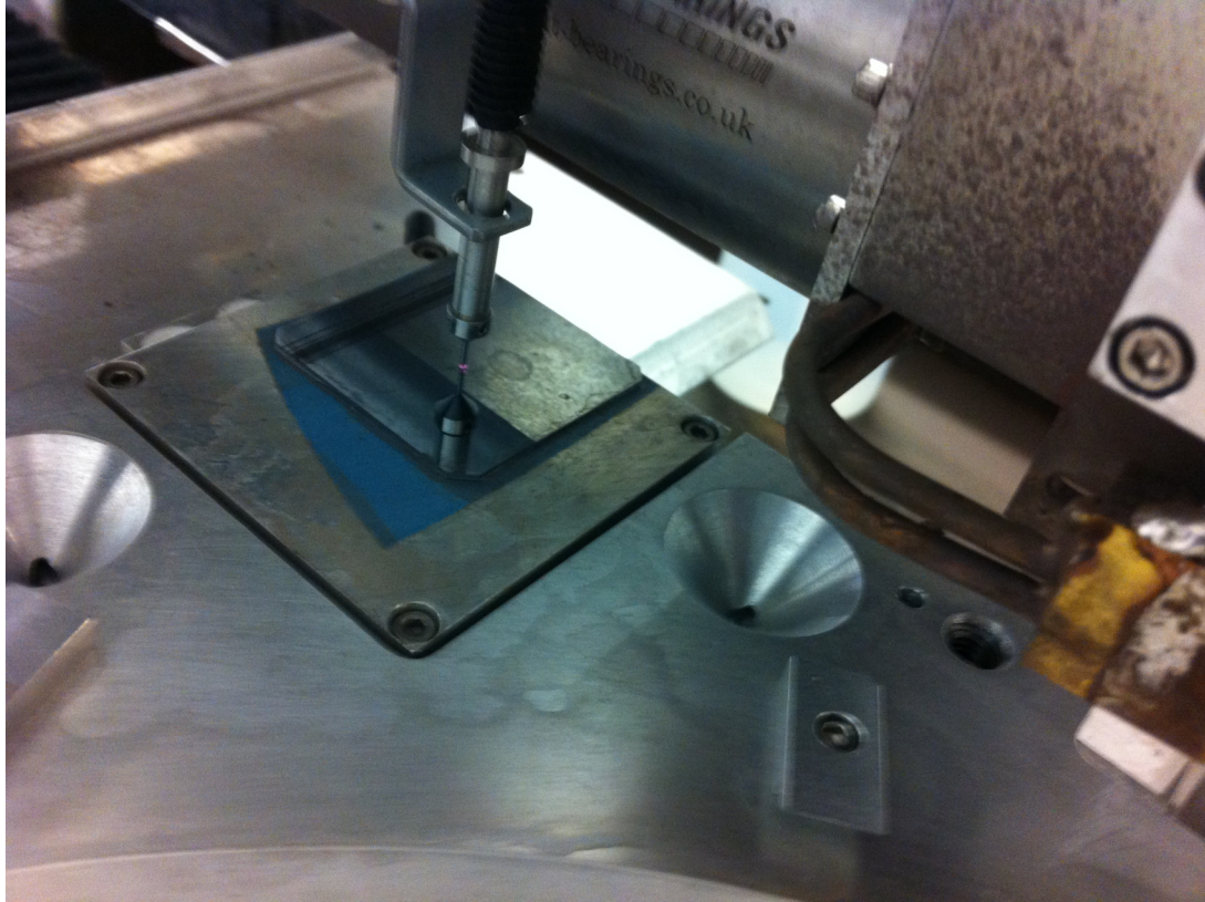
Figure 4.5: The measurement gauge mounted next to the spindle and engaged in measuring a silicon test wafer. The 1mm spherical ruby tip is visible in red in the center of the picture. This gauge provided sub-micron measurement repeatability.
