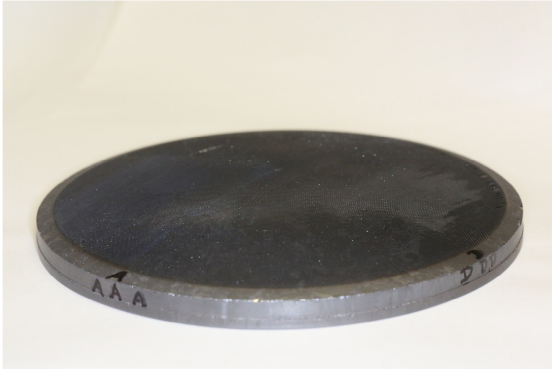
Figure 4.24: A polycrystalline silicon lens mockup. This piece was a mechanical blank from an earlier stage of the ACT project, and was used as a demonstration piece for cutting a curved surface. A single structured layer was cut into the surface successfully. There is a small amount of chipping along one edge due to the polycrystalline material being weak enough along grain boundaries to flake apart from the force of cutting. This problem was not observed in actual optics consisting of monocrystalline silicon.
