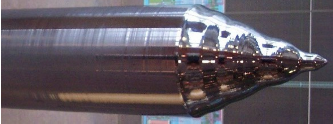
Figure 3.1: A single-crystal boule of silicon. Boules like this are generated by pulling molten silicon using a seed crystal (either via float zone or Czochralski processes, depending on desired size and required purity - Czochralski achieving larger sizes, but introducing oxygen impurities due to the silica crucibles used in processing). Image used under the creative commons license [11].
