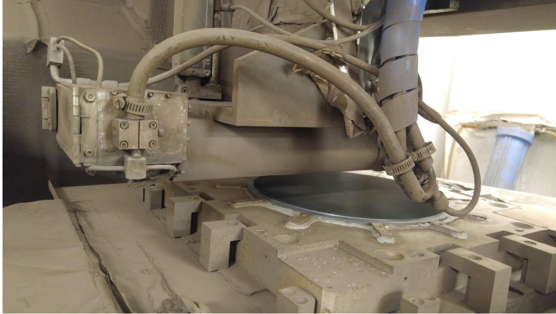
Figure 4.7: The dicing spindle, mounted to the Z-stage interface plate and covered in the hard-earned dirt from many successfully cut optics.
