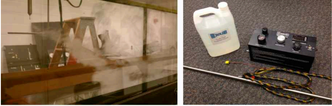
Figure 3.6: Example smoke plume made by the smoke generator system on right.
