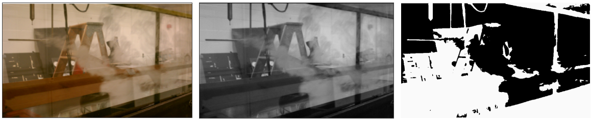
Figure 3.10: The filtering of a color image of the smoke plume, to greyscale, to black-and-white.
