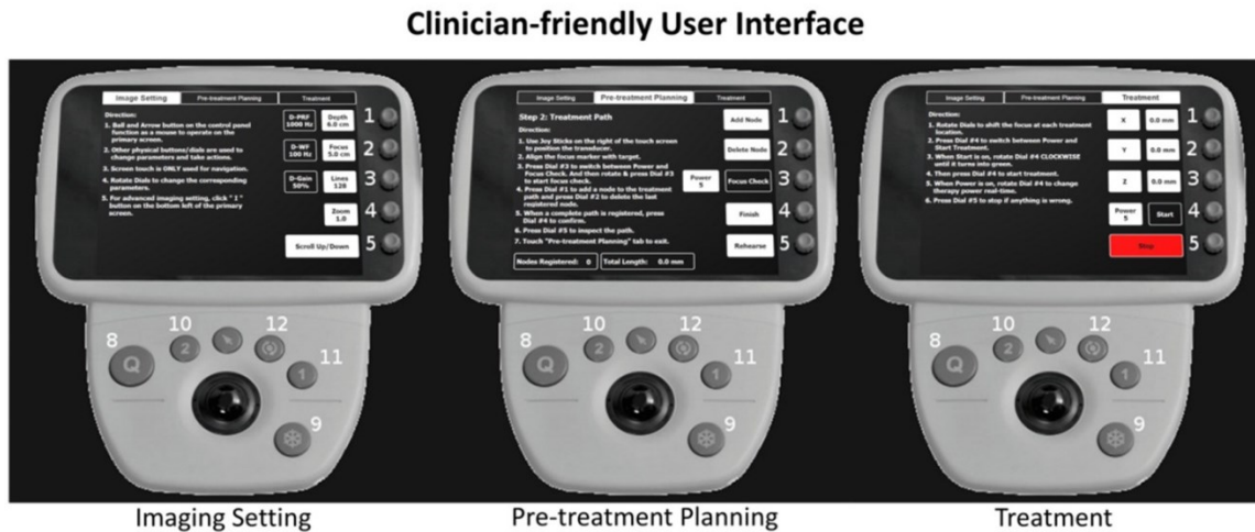
Figure 2.14: Control panel with a touch screen and physical buttons and knobs, with different touch screen interfaces shown. There are tabs: one for imaging setting, one for pre-treatment planning and one for treatment. Detailed operation instructions are listed on the left of each tab.
