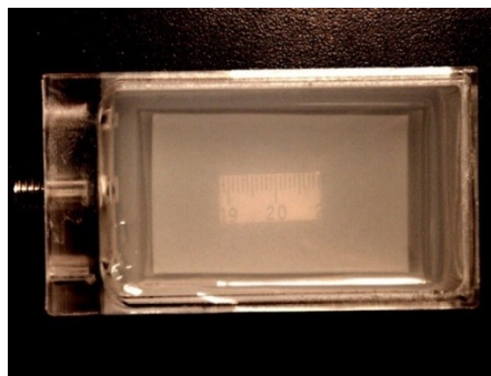
Figure 6.1: Transparent fibrin clot embedded in agarose hydrogel. The clot was molded to be rectangular in shape. A ruler segment was placed under the clot to show the transparency.
