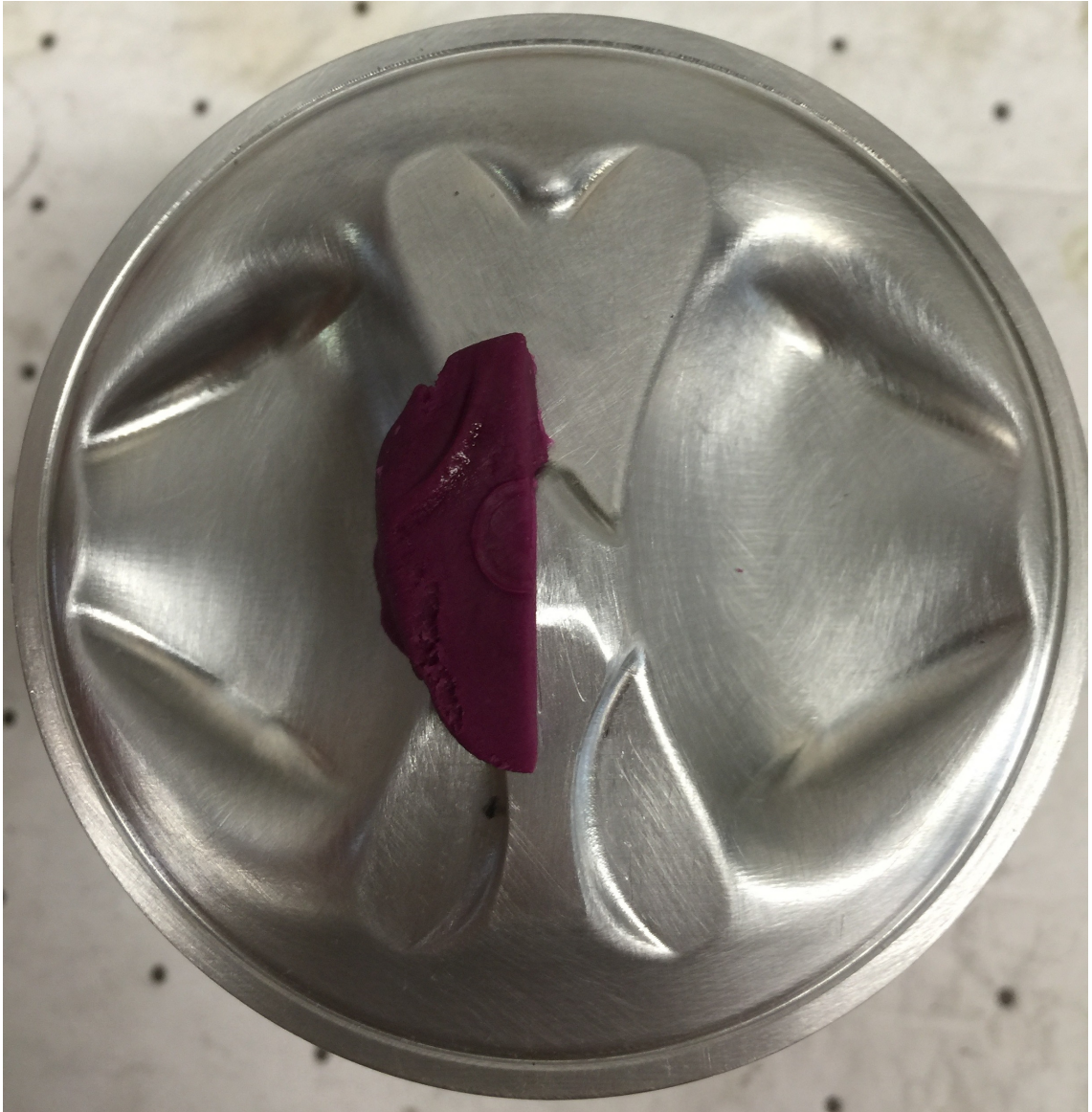
Figure 4.11: Top view of the Zeta prototype piston geometry with modeling clay used for checking injector, valve, and combustion chamber dome clearancing.
