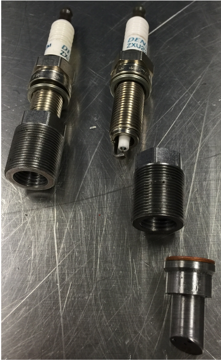
Figure 4.6: Spark plugs, pre-chamber retention nuts, and pre-chamber insert.
