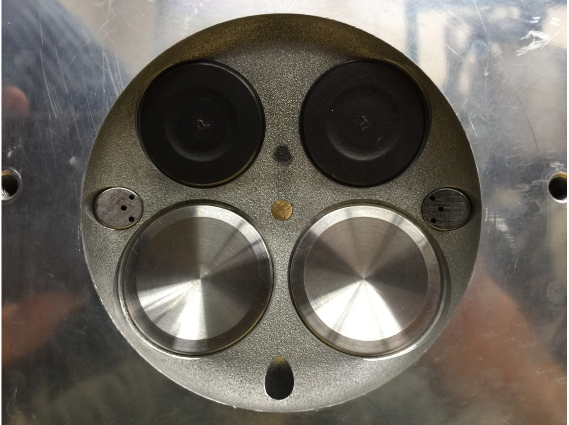
Figure 4.8: Combustion chamber dome featuring the pre-chamber location at the 3 o'clock and 9 o'clock positions. The 6 o'clock shadow is the pressure transducer port. A brass plug is installed in the center, where the direct injector is installed.
