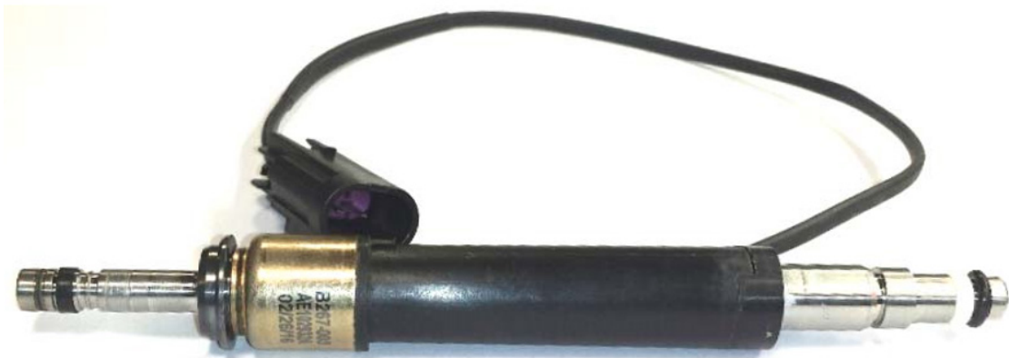
Figure 4.17: One physical example of the custom Delphi fuel injectors created for the DPC Zeta prototype engine.
