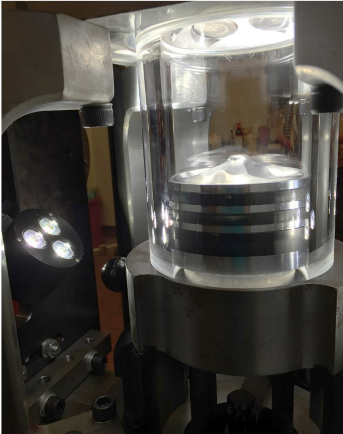
Figure 4.3: The fully transparent cylinder liner installed in the Zeta prototype engine and illuminated using the LED lighting system.
