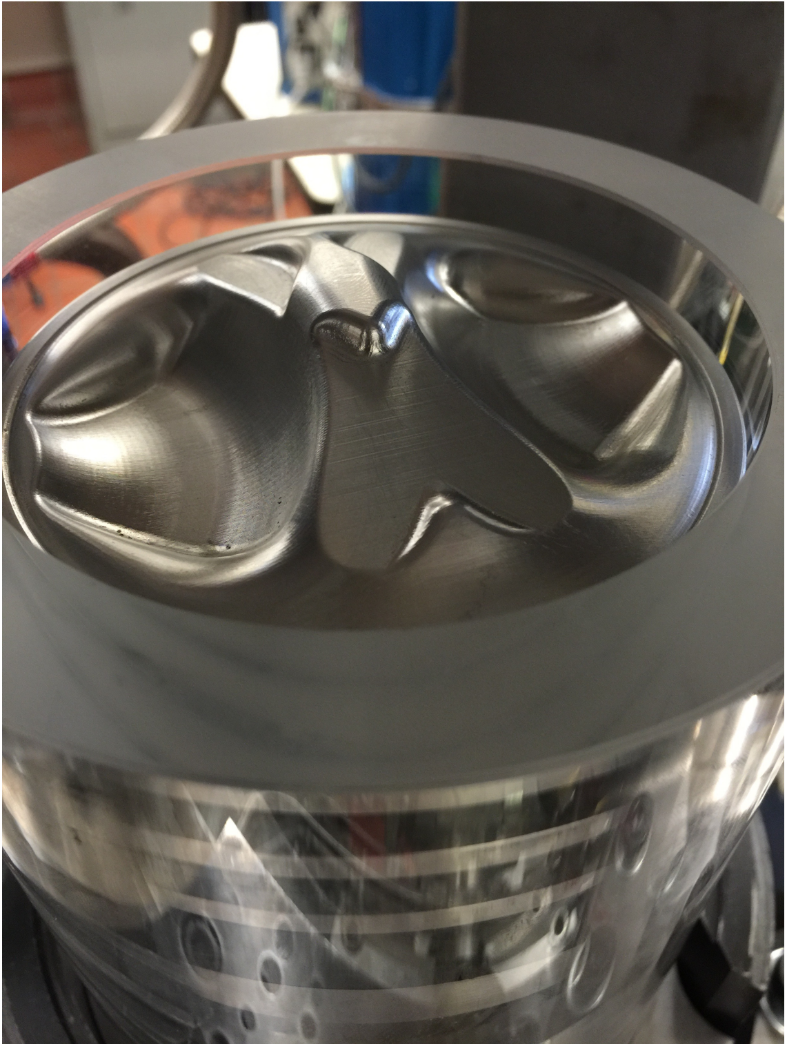
Figure 4.10: Profile close-up view of the Zeta prototype piston geometry installed in the optical liner with the Torlon compression rings.
