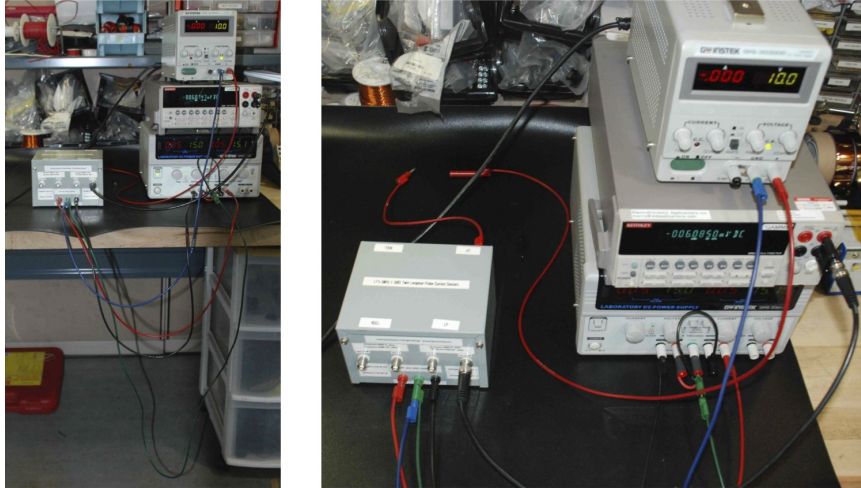
Figure B.7: Pictures of the equipment setup for calibrating the Dual-Symmetric Current Sensing Circuit
