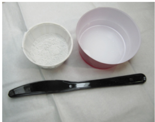
Figure B.3: Picture on the left: The components of the Ceramabond mixture, 571-L and 571-P. Picture on the right: 571-P in the small paper cup, and 571-L in the red cup before mixing.
