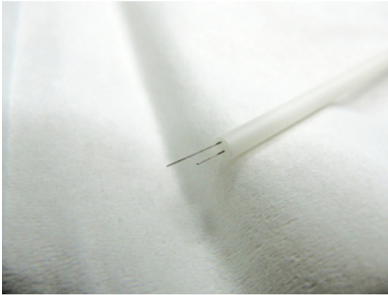
Figure B.2: Picture on the left: The top of the Langmuir probe showing the lengths allotted for the LP and Null probes. Picture on the right: The back of the Langmuir probe showing the Null and LP wires insulated from each other and held in place in the alumina tube using Kapton tape.
