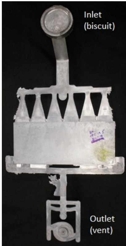
Figure 2.1: Plate casting geometry, where the metal enters the die at the top, and exits at the bottom. This includes the biscuit and vacuum structure.
