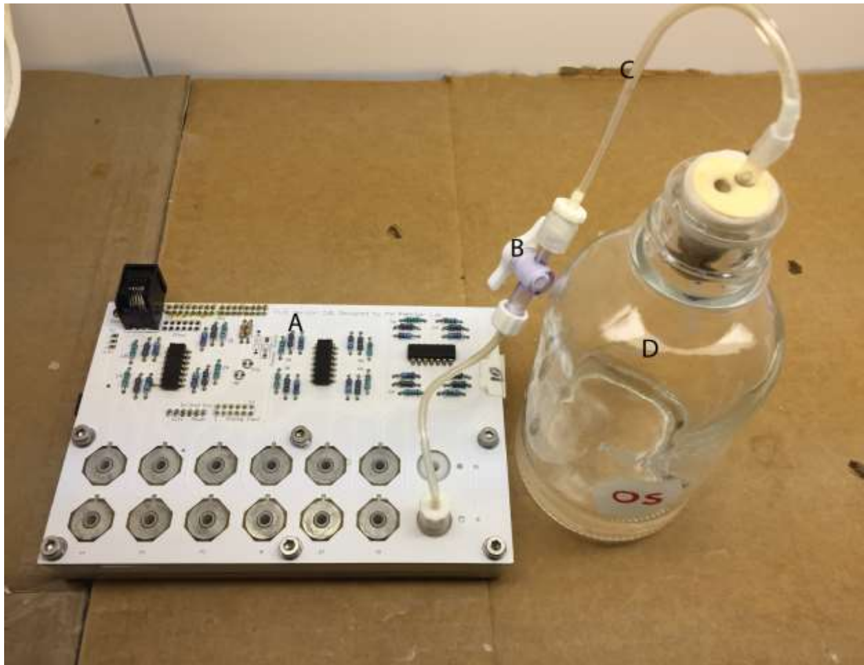
Fig. 2. 2. Photo of the reservoir system for long term FLIC.
