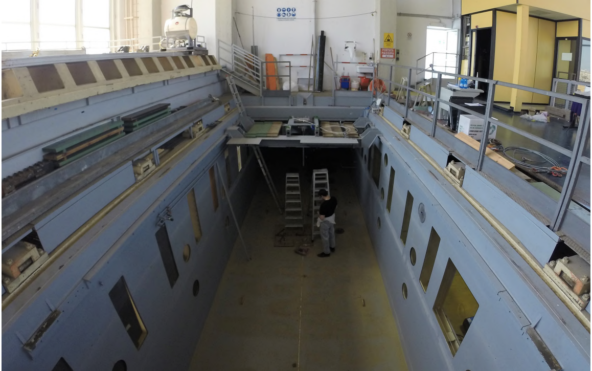
(a) View from downstream end of the INSEAN tunnel section. The hydrofoil is visible near the center of the frame. The channel lid is the large beige structure visible on the left-hand side of the frame.
