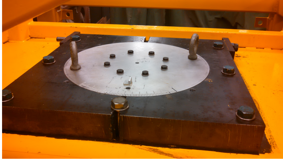
Figure 2.11: Rotating disk and clamp used to set yaw angle of hydrofoil. The disk rotates about the Z-axis of the hydrofoil shown in figure 2.9. The disk is machined from aluminum, while the clamp is machined from mild steel. A horizontal threaded rod on the opposite side of the clamp is used to apply clamping pressure around the circumference of the disk. Four additional flanged bolts are threaded into the tapped holes visible in the clamp, distributed around the disk's circumference, which apply a vertical clamping force to keep the constrain the vertical orientation of the hydrofoil.
