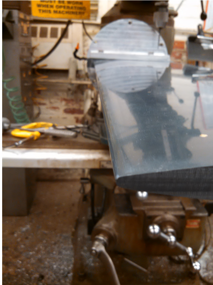
Figure 2.6: Photo of surface-finish of PVC hydrofoil after LE treatment and polishing.
