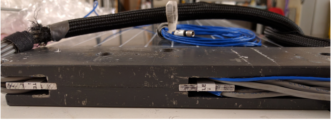
Figure 2.29: Photo of spars inserted into flexible hydrofoil until flush with the mounting tang.
