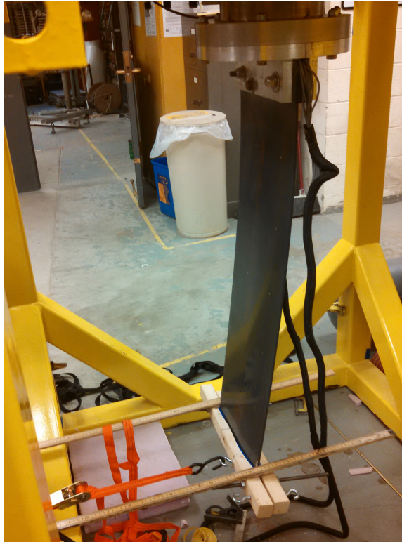
(a) Loads being applied to the hydrofoil during calibration. The tension is being applied forward of the elastic axis, leading to a combined bending and twisting response.
