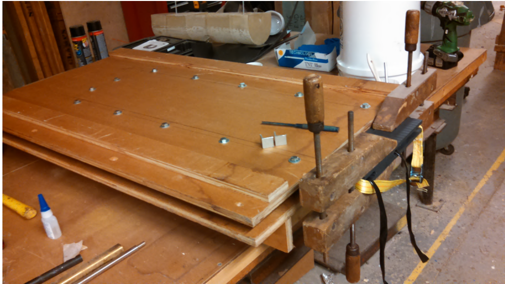
Figure 2.5: Photo of PVC hydrofoil being clamped during chemical weld.
