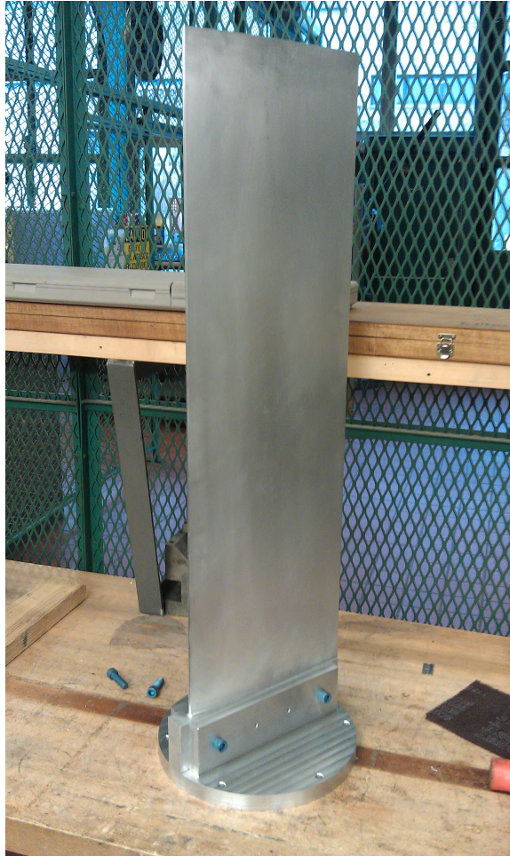
Figure 2.3: Photo of aluminum hydrofoil (Model 0), prior to hardcoat anodizing.
