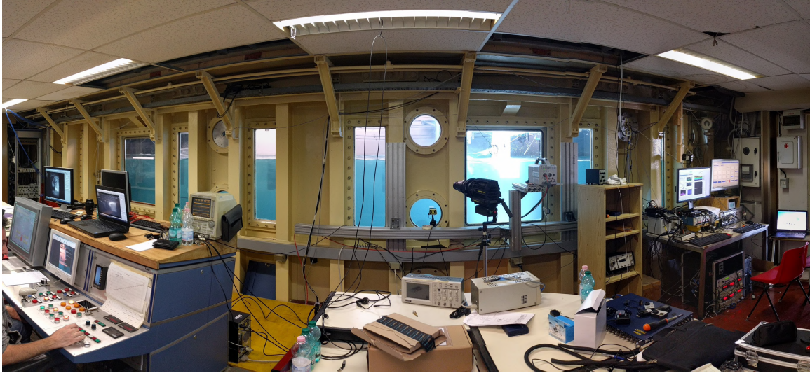
Figure 2.17: Photo of control room and observation windows at CNR-INSEAN recirculating water channel. All control of tunnel speed and pressure, data acquisition, signal generation, and videography were performed inside of the control room.
