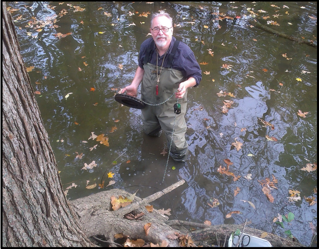
Figure 10. Robert Muller holding the PVC casing with the temperature sensor inside and the break rotor.
