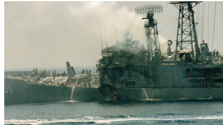
Figure 22: AIREX Damage to USS Stark
