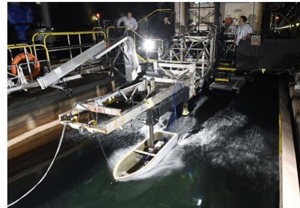
Figure 18: Planing boat test at NSWCCD
