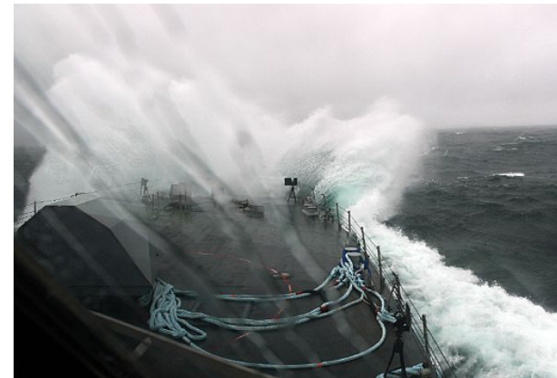
Figure 19: USS For Worth Bow Flare Impact
