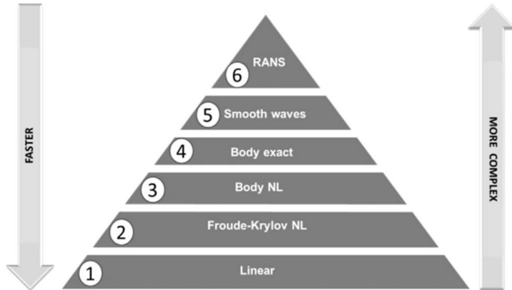
Figure 3: Hydrodynamic methods. Taken from P. Temarel et al., Report of Committee I.2 Loads, 17th International Ships and Offshore Structures Congress , 16-21 August 2009, Seoul, South Korea, Volume I, Pages 127—210
