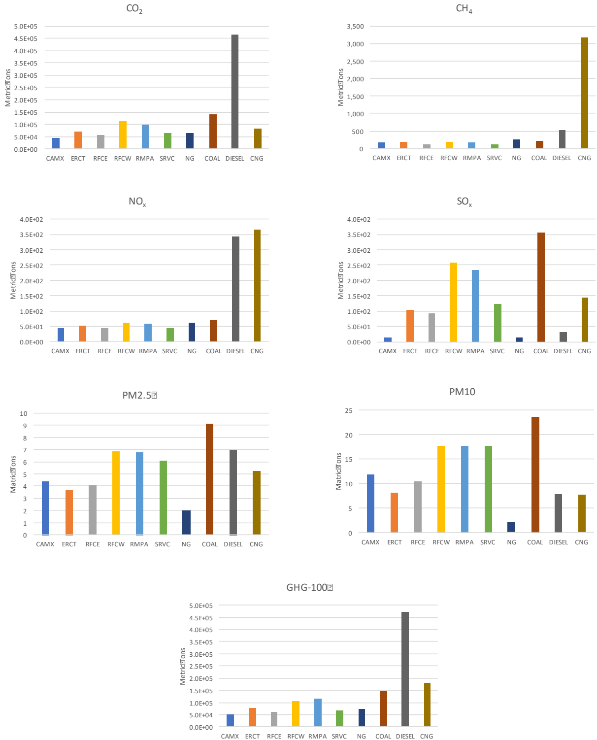
Figure 5: Lifetime electricity lifecycle emissions for electric baggage tractors and fuel cycle emissions (upstream and combustion) emissions LS diesel and CNG baggage tractors.
