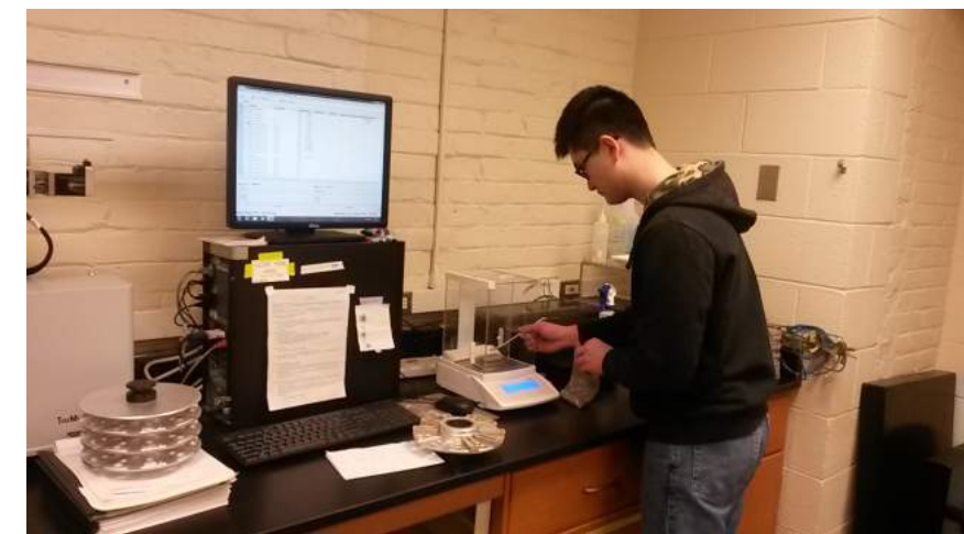
Preparing soil samples to analyze via the LECO determinator.
