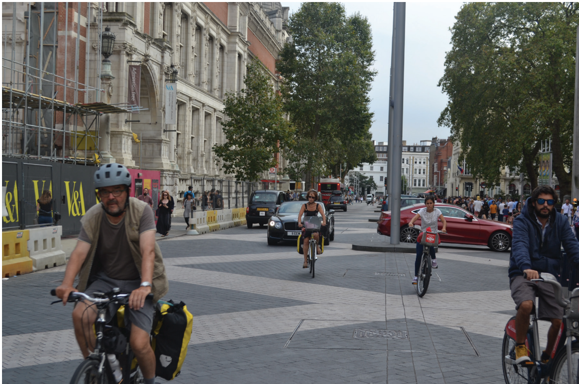
Figure 4-23: While pedestrians are unwilling to compete with vehicles in Zone 2, bicyclists do share the travelway and the flat, continuous surface of the shared street design gives them additional room for maneuvering.
