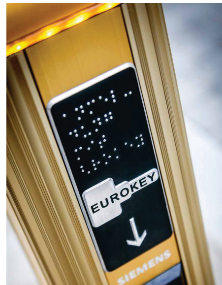
Figure 5-14: The Euro-Key allows the visually impaired to activate a cross walk in the shared street zones. Source: Christian Fürthner
