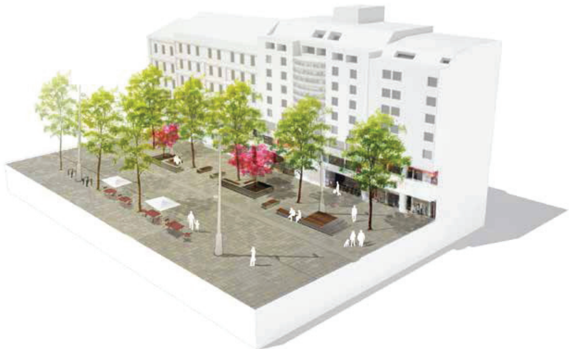
Figure 5-10: This schematic axonometric section shows the structure of the street, with an asymmetric travelway, ample transitional seating areas, and a wide pedestrian safe zone along the building facade. Source: Bureau B+B.
