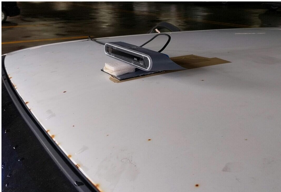
Figure 4-9: Illustration showing the ZED camera installation for the car experiment.
