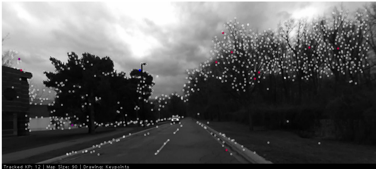
Figure 4-10: Illustration showing a frame from the car sequence where the VO algorithm fails.
