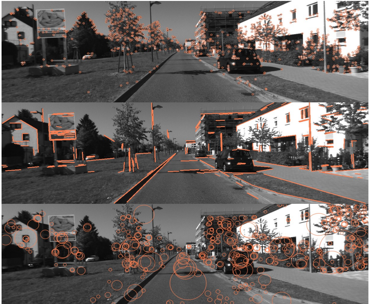
Figure 2-8: Common feature types: [TOP] Points or corners, [MIDDLE] Lines, [BOTTOM] Blob or region features.
