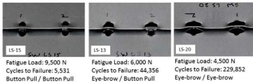
Figure 2.5. Typical failure mode of steel-steel SW
