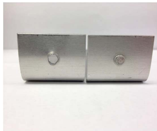
(b) Button pull failure
